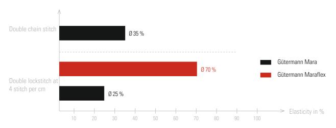
Maraflex was specifically developed for the use on both lockstitch and chain stitch machines when stitching highly elastic fabrics. Maraflex is the reliable partner when it comes to lockstitch operations as Maraflex is ideally suited to both upper and bobbin thread. In addition highly elastic decorative seams are possible without compromising the appearance.
